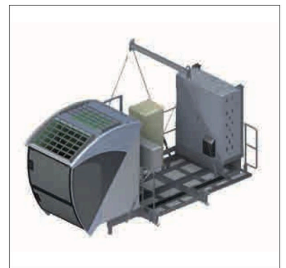
New cabin platform design with wide access to the counter-jib and resistor for better cable management
