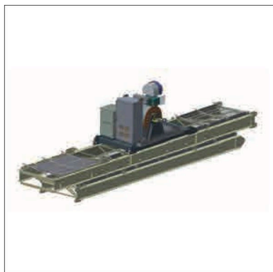
New counter-jib design with quick engagement for easy maintenance and transportation
