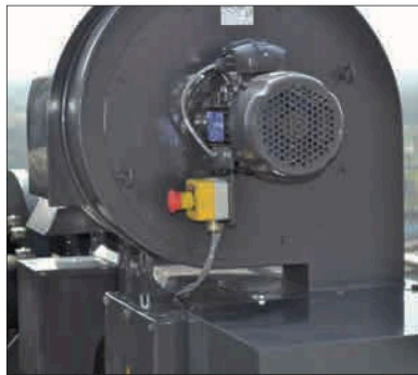
Emergency push button within operator reach when monitoring and maintaining the crane
